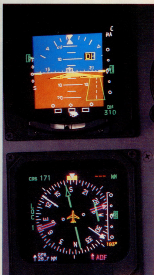
The Caution and Warning System (CAWS) panel includes annunciators for Pusher Ice Mode and other system alerts (left). With the EFS 40/50 (below, shown with a localizer frequency as primary navigation) plus a mechanical RMI, there are plenty of ways to navigate. The AOA indicator is at left edge of the EADI. A pictorial "runway" shows your position in the EADI's localizer mode.
