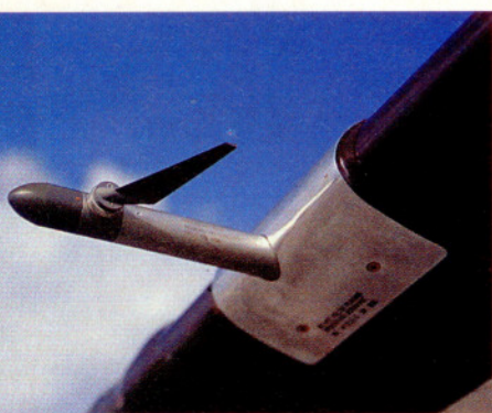
Angle-of-attack probes—one on each wing—send information to the stick shaker-pusher system. Probe anti-ice must be on for every flight. The probe, AOA vane, and mounting plate are all heated.
